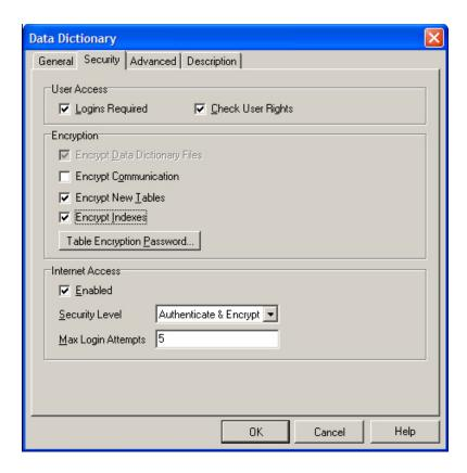
Another security enhancement is the option to encrypt client-server communication on local networks. Prior to this release, only those clients connecting to ADS over the Internet had an option to employ encrypted communication. You use the Encrypt Communication check box shown in Figure 3 to enable this feature.
